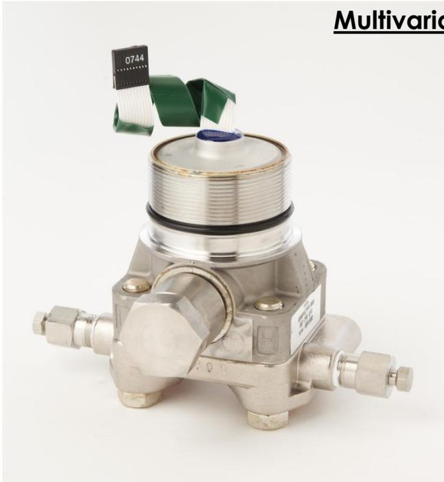
The Multivariable Sensor is a 3-in-1 model 205 transmitter manufactured by Rosemount® Inc. for Dynamic Flow Computers. This sensor measures static/ absolute pressure, differential pressure, and using an optional RTD, process temperature. These three process variables are available all the time and updates are sent to the flow computer up to NINE times per second.
